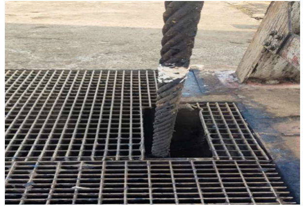
Worn out steel wire rope of Scour Vent Gate
